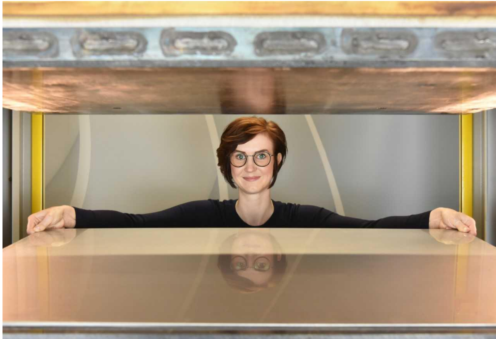
Image caption: Award-winner Dr.-Ing. Larissa Born loading the mirror plates (tool for the for the production of test specimens) into the hot press ©DITF Denkendorf
